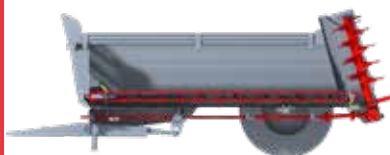
Drive line with transmission under the lowered axle (ideal for sloping terrain).
